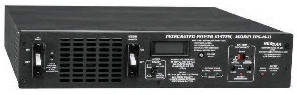
interruption in the event of AC loss. Batteries are recharged when AC is restored. A manual battery disconnect switch allows internal or external battery service or replacement while the system is running.
