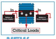
It automatically selects the higher voltage of two independent DC power sources and routes that source to the load. Should one source falter or fail, the other will automatically supply the load with no transfer delay, thus operation continues uninterrupted.
